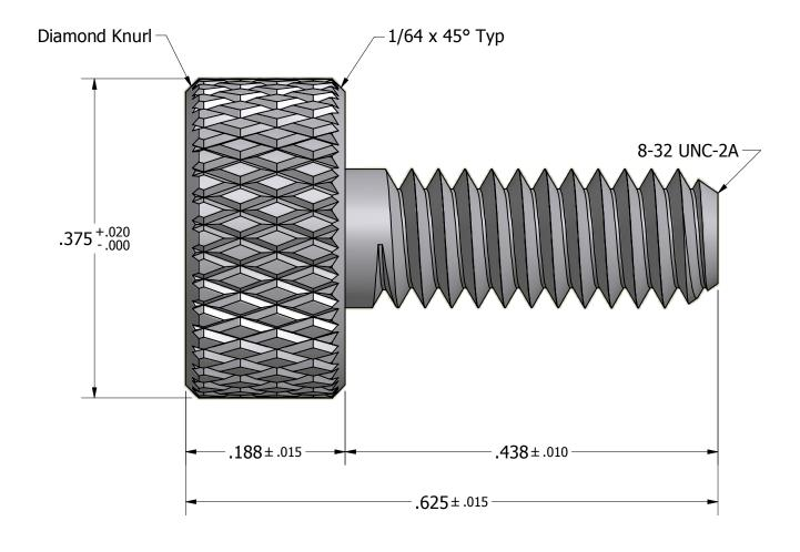
Tolerances Unless Otherwise Specified: **LYN-TRON, INC.** .xx Decimal: ± .02 .xxx Decimal: ± .005 Part Number: Fraction: ± 1/64 ± 2° ST7629 Angle: Description: **Plain Thumb Screw** Drawn By: Gauge: Material: Scale: COURTNEYS09/11/2012 Steel 9:1
