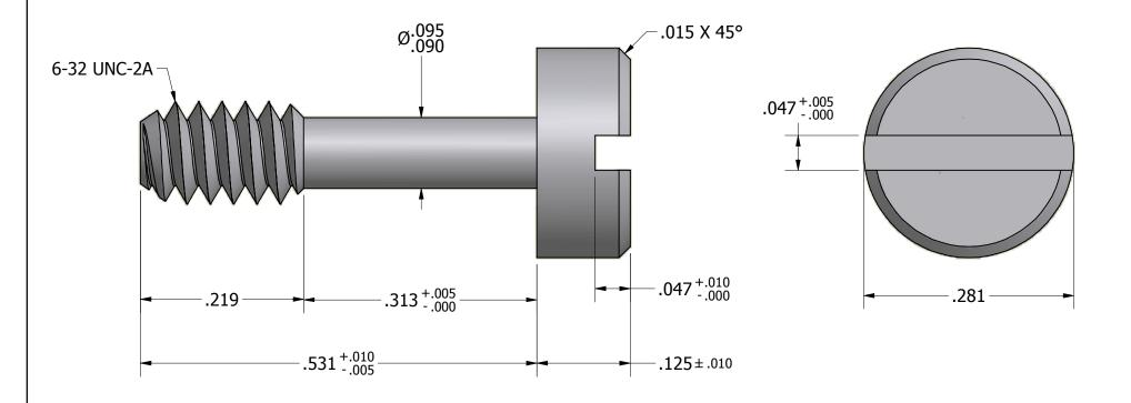
Tolerances Unless Otherwise Specified: **LYN-TRON, INC.** .xx Decimal: ± .02 .xxx Decimal: ± .005 Part Number: Fraction: ± 1/64 ± 2° ST7585 Angle: Description: **Captive Panel Screw -- Type 6** Material: Drawn By: Gauge: Scale: **JEFFN** 06/12/2012 7:1 Steel
