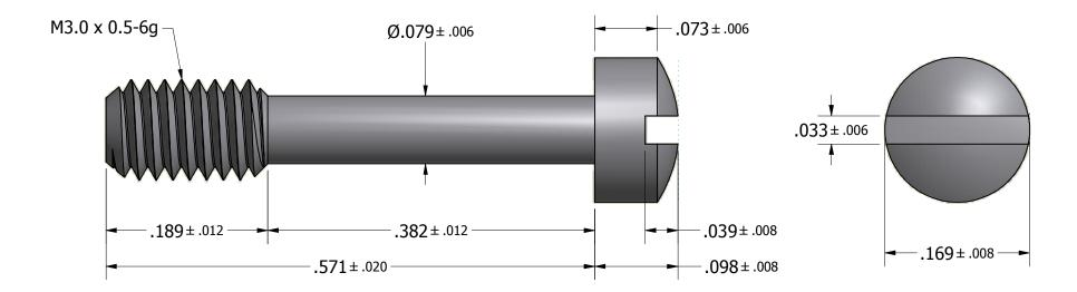
Tolerances Unless Otherwise Specified: **LYN-TRON, INC.** .xx Decimal: ± .01 .xxx Decimal: ± .004 Part Number: Fraction: ± 1/64 ± 2° ST5788 Angle: Description: 4.3mm Rnd Captive Panel Screw -- Type 4 Drawn By: Material: Gauge: Scale: Cameron C. 1/14/2014 **Stainless Steel** 8:1
