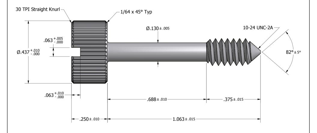
Tolerances Unless Otherwise Specified: **LYN-TRON, INC.** .xx Decimal: ± .02 .xxx Decimal: ± .005 Fraction: ± 1/64 ± 2° ST3145 Angle: Description: **Captive Panel Screw -- Type 1** Drawn By: Material: Gauge: Scale: COURTNEYS03/01/2011 Steel 5:1
