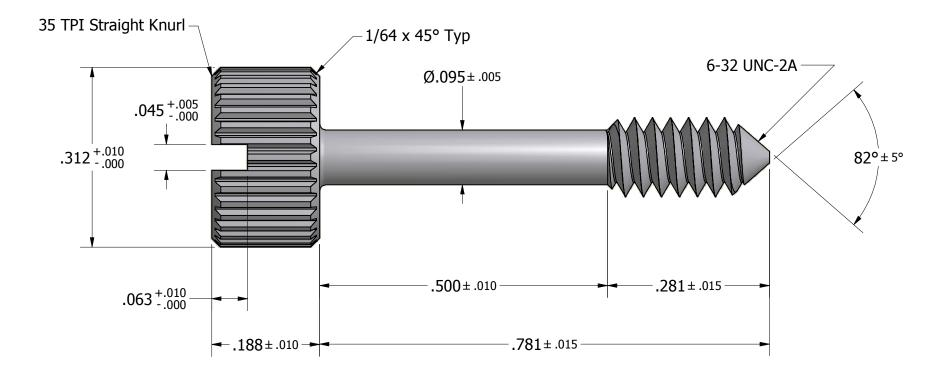
Tolerances Unless Otherwise Specified: **LYN-TRON, INC.** .xx Decimal: ± .02 .xxx Decimal: ± .005 Part Number: Fraction: ± 1/64 ± 2° ST3107 Angle: Description: **Captive Panel Screw -- Type 1** Drawn By: Material: Gauge: Scale: COURTNEYS02/09/2011 Steel 6:1
