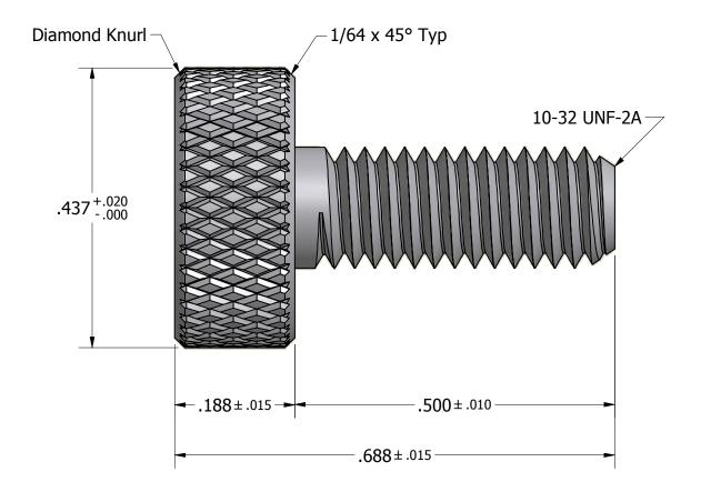
Tolerances Unless Otherwise Specified: **LYN-TRON, INC.** .xx Decimal: ± .02 .xxx Decimal: ± .005 Part Number: Fraction: ± 1/64 ± 2° SS7635 Angle: Description: **Plain Thumb Screw** Drawn By: Gauge: Material: Scale: COURTNEYS09/11/2012 **Stainless Steel** 9:1
