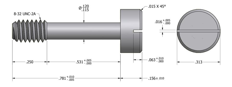
Tolerances Unless Otherwise Specified: **LYN-TRON, INC.** .xx Decimal: ± .02 .xxx Decimal: ± .005 Part Number: Fraction: ± 1/64 ± 2° SS7590 Angle: Description: **Captive Panel Screw -- Type 6** Drawn By: Material: Gauge: Scale: COURTNEYS09/06/2012 **Stainless Steel** 6:1
