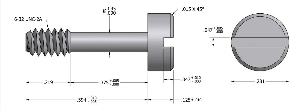
Tolerances Unless Otherwise Specified: **LYN-TRON, INC.** .xx Decimal: ± .02 .xxx Decimal: ± .005 Part Number: Fraction: ± 1/64 ± 2° **SS7586** Angle: Description: **Captive Panel Screw -- Type 6** Material: Drawn By: Gauge: Scale: **JEFFN** 06/12/2012 7:1 **Stainless Steel**
