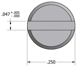
Tolerances Unless Otherwise Specified: **LYN-TRON, INC.** .xx Decimal: ± .02 .xxx Decimal: ± .005 Part Number: Fraction: ± 1/64 ± 2° SS7584 Angle: Description: **Captive Panel Screw -- Type 6** Material: Drawn By: Gauge: Scale: **JEFFN** 06/12/2012 **Stainless Steel** 7:1
