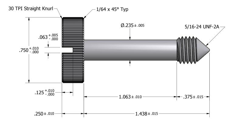
Tolerances Unless Otherwise Specified: **LYN-TRON, INC.** .xx Decimal: ± .02 .xxx Decimal: ± .005 Part Number: Fraction: ± 1/64 SS3357 Angle: ± 2° Description: **Captive Panel Screw -- Type 1** Drawn By: Material: Gauge: Scale: COURTNEYS02/22/2011 **Stainless Steel** 1:1
