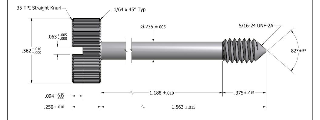
Tolerances Unless Otherwise Specified: **LYN-TRON, INC.** .xx Decimal: ± .02 .xxx Decimal: ± .005 Part Number: Fraction: ± 1/64 ± 2° SS3342 Angle: Description: **Captive Panel Screw -- Type 1** Drawn By: Material: Gauge: Scale: COURTNEYS02/22/2011 NTS **Stainless Steel**
