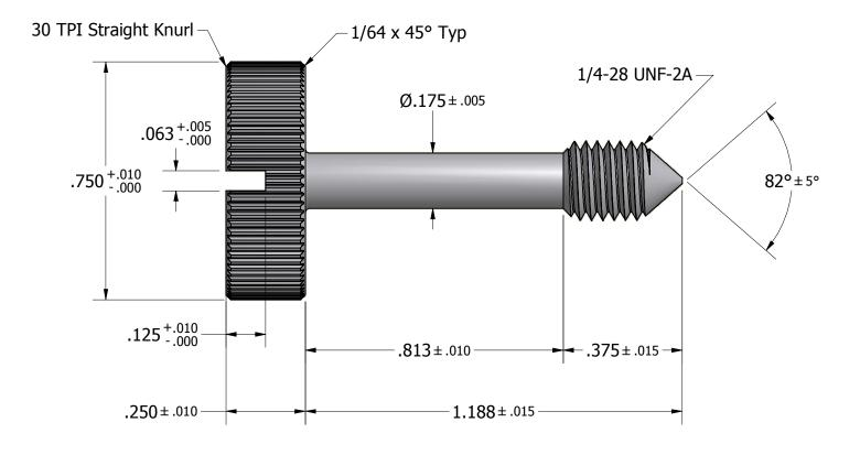
Tolerances Unless Otherwise Specified: **LYN-TRON, INC.** .xx Decimal: ± .02 .xxx Decimal: ± .005 Part Number: Fraction: ± 1/64 SS3285 Angle: ± 2° Description: **Captive Panel Screw -- Type 1** Drawn By: Material: Gauge: Scale: COURTNEYS02/22/2011 **Stainless Steel** 4:1
