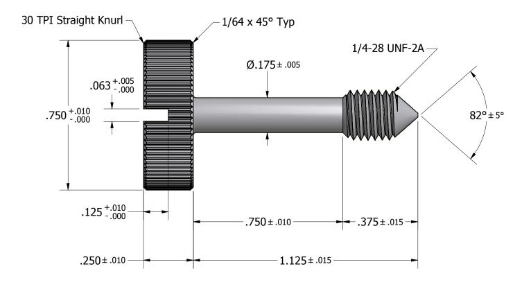
Tolerances Unless Otherwise Specified: **LYN-TRON, INC.** .xx Decimal: ± .02 .xxx Decimal: ± .005 Part Number: Fraction: ± 1/64 SS3284 Angle: ± 2° Description: 3/4 Rd SS CPS type 1(1.375) Drawn By: Material: Gauge: Scale: COURTNEYS02/22/2011 **Stainless Steel** 5:1
