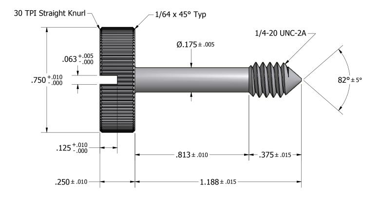
Tolerances Unless Otherwise Specified: **LYN-TRON, INC.** .xx Decimal: ± .02 .xxx Decimal: ± .005 Part Number: Fraction: ± 1/64 SS3239 Angle: ± 2° Description: **Captive Panel Screw -- Type 1** Drawn By: Material: Gauge: Scale: COURTNEYS02/22/2011 **Stainless Steel** 4:1
