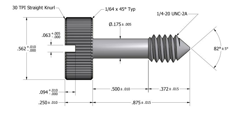
Tolerances Unless Otherwise Specified: **LYN-TRON, INC.** .xx Decimal: ± .02 .xxx Decimal: ± .005 Part Number: Fraction: ± 1/64 ± 2° SS3211 Angle: Description: **Captive Panel Screw -- Type 1** Drawn By: Material: Gauge: Scale: COURTNEYS02/22/2011 **Stainless Steel** 5:1
