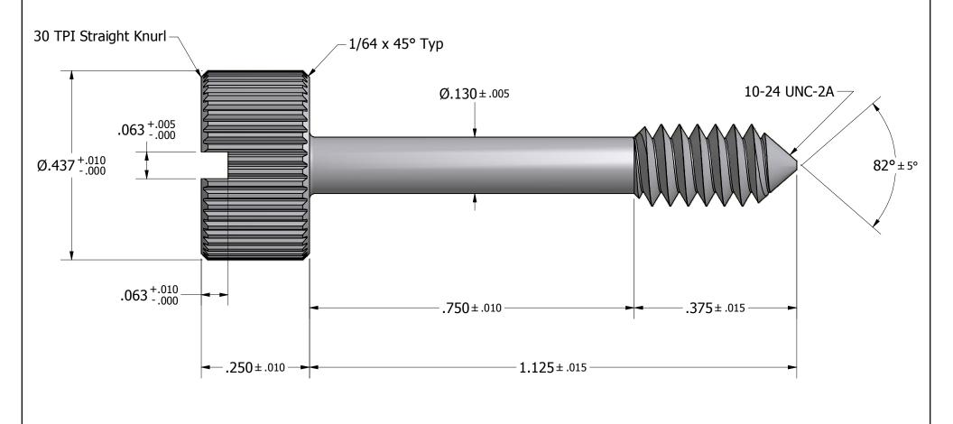
Tolerances Unless Otherwise Specified: **LYN-TRON, INC.** .xx Decimal: ± .02 .xxx Decimal: ± .005 Part Number: Fraction: ± 1/64 ± 2° SS3146 Angle: Description: **Captive Panel Screw -- Type 1** Drawn By: Material: Gauge: Scale: COURTNEYS02/22/2011 **Stainless Steel** 5:1
