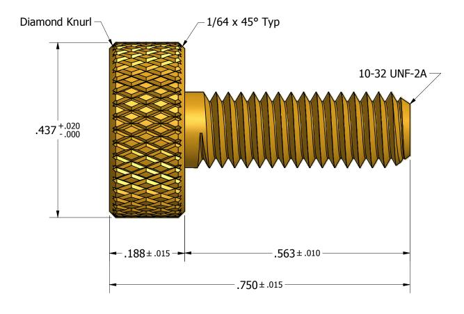
Tolerances Unless Otherwise Specified: **LYN-TRON, INC.** .xx Decimal: ± .02 .xxx Decimal: ± .005 Part Number: Fraction: ± 1/64 ± 2° **BR7636** Angle: Description: **Plain Thumb Screw** Drawn By: Gauge: Material: Scale: COURTNEYS09/11/2012 7:1 **Brass**
