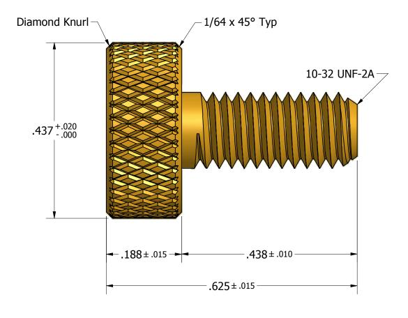
Tolerances Unless Otherwise Specified: **LYN-TRON, INC.** .xx Decimal: ± .02 .xxx Decimal: ± .005 Part Number: Fraction: ± 1/64 ± 2° **BR7634** Angle: Description: **Plain Thumb Screw** Drawn By: Gauge: Material: Scale: COURTNEYS09/11/2012 **Brass** 9:1
