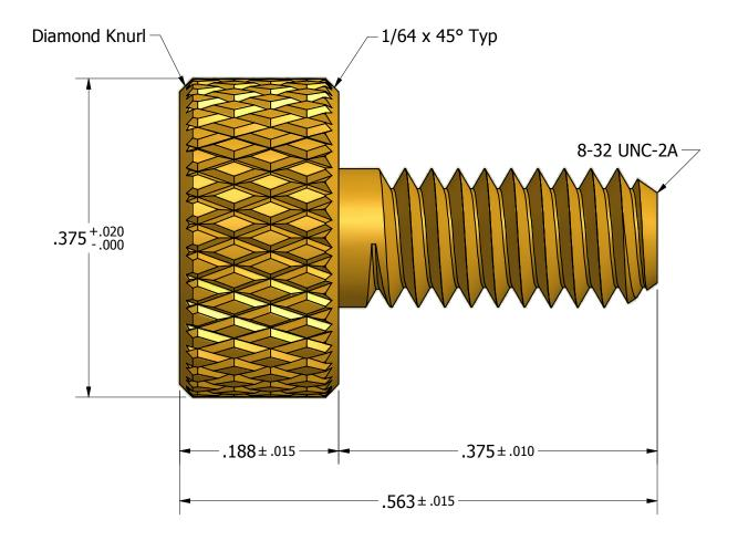
Tolerances Unless Otherwise Specified: **LYN-TRON, INC.** .xx Decimal: ± .02 .xxx Decimal: ± .005 Part Number: Fraction: ± 1/64 ± 2° **BR7628** Angle: Description: **Plain Thumb Screw** Drawn By: Gauge: Material: Scale: COURTNEYS09/11/2012 **Brass** 9:1
