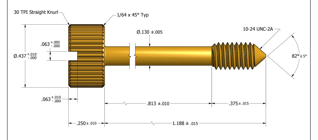
Tolerances Unless Otherwise Specified: **LYN-TRON, INC.** .xx Decimal: ± .02 .xxx Decimal: ± .005 Fraction: ± 1/64 ± 2° **BR3147** Angle: Description: **Captive Panel Screw -- Type 1** Drawn By: Material: Gauge: Scale: COURTNEYS02/09/2011 NTS **Brass**
