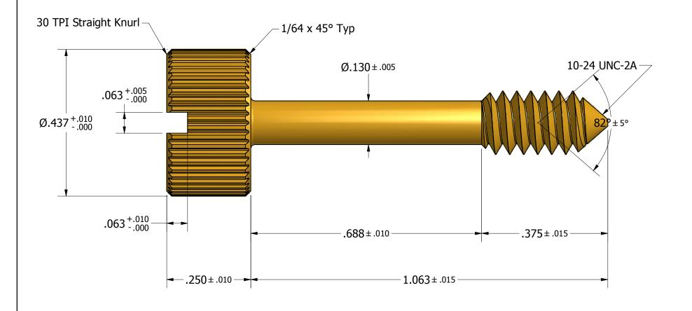
Tolerances Unless Otherwise Specified: **LYN-TRON, INC.** .xx Decimal: ± .02 .xxx Decimal: ± .005 Fraction: ± 1/64 ± 2° **BR3145** Angle: Description: **Captive Panel Screw -- Type 1** Drawn By: Material: Gauge: Scale: COURTNEYS02/09/2011 **Brass** 5:1
