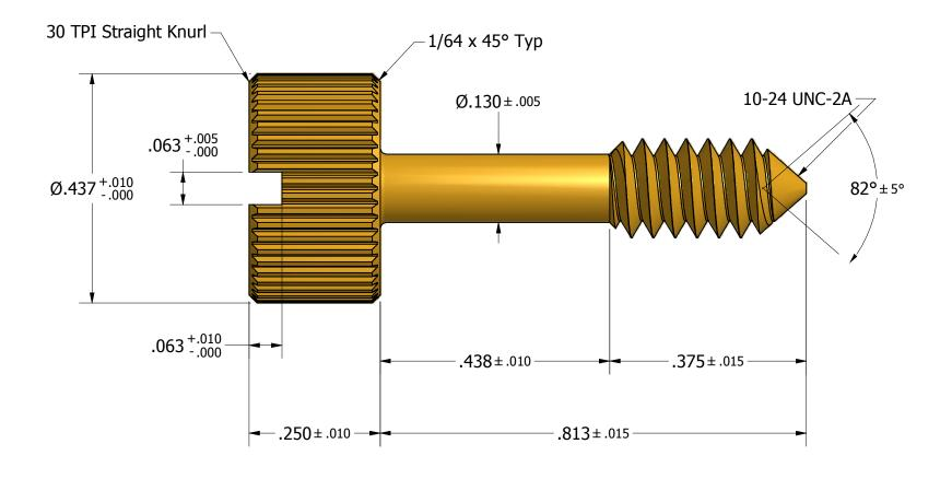
Tolerances Unless Otherwise Specified: **LYN-TRON, INC.** .xx Decimal: ± .02 .xxx Decimal: ± .005 Fraction: ± 1/64 ± 2° **BR3141** Angle: Description: **Captive Panel Screw -- Type 1** Drawn By: Material: Gauge: Scale: COURTNEYS02/09/2011 **Brass** 6:1
