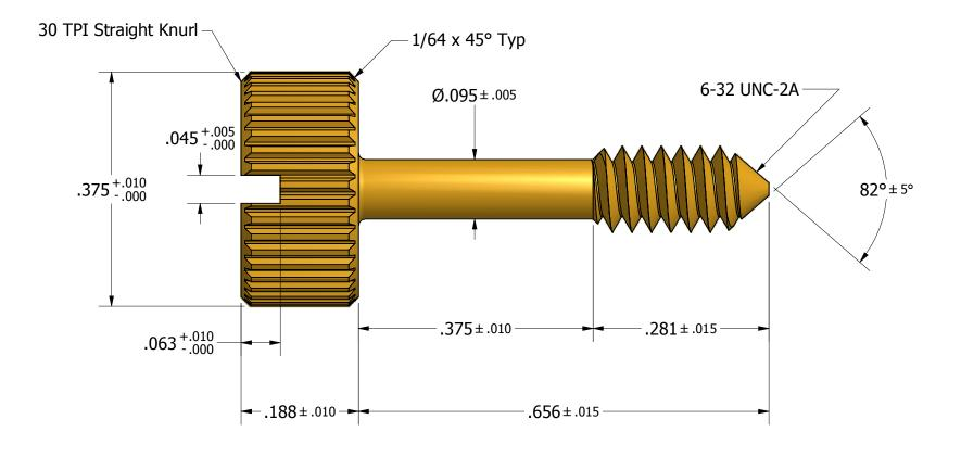
Tolerances Unless Otherwise Specified: **LYN-TRON, INC.** .xx Decimal: ± .02 .xxx Decimal: ± .005 Part Number: Fraction: ± 1/64 ± 2° **BR3110** Angle: Description: 3/8 Rd 632 CPS type 1 (.843) Drawn By: Material: Gauge: Scale: COURTNEYS02/09/2011 **Brass** 6:1
