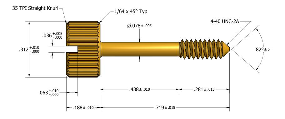
Tolerances Unless Otherwise Specified: **LYN-TRON, INC.** .xx Decimal: ± .02 .xxx Decimal: ± .005 Part Number: Fraction: ± 1/64 ± 2° **BR3101** Angle: Description: **Captive Panel Screw -- Type 1** Drawn By: Material: Gauge: Scale: COURTNEYS02/09/2011 **Brass** 6:1
